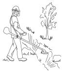
5 Take great care when cutting a tree that is in tension. A tree that is in tension may spring back to its normal position before or after being cut. If you position yourself incorrectly or make the cut in the wrong place the tree may hit you or the machine and cause you to lose control. Both situations can cause serious personal injury.
